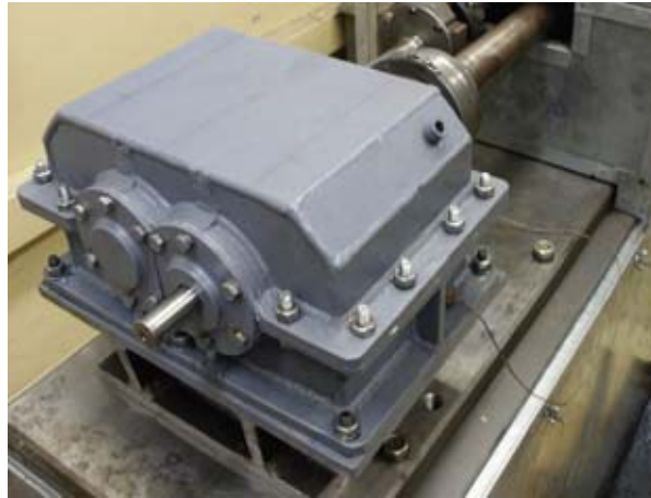
Fig. 1. View of the gear tested on the FZG power circulating stand
